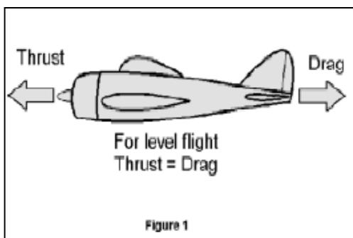
Drag, like lift is measured in pounds. Gravity always pulls our plane down, Drag always pulls our plane back. The engine that makes our plane
