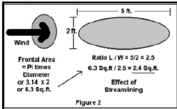
The drag Coefficient and the conversion factors are all included in the number .0033. Plugging in the numbers above we find the force on a 1 sq. foot plate at 40 m.p.h. is  $.0033 \times 1 \times 40 \times 40$ . This comes out to 5.3 pounds.
