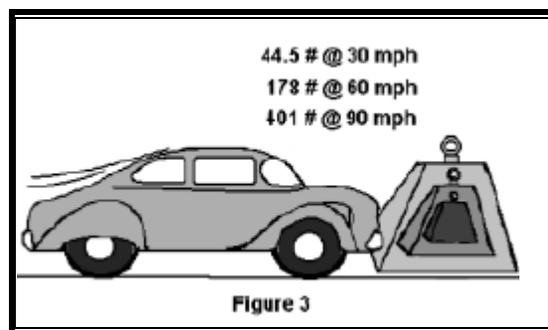
Because the car is somewhat streamlined, much more air leaks past it so the "effective" board area is less than 30 Sq. ft. A small car is about half as wide as it is long, so let's reduce our frontal area by 2.
