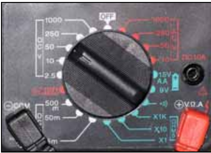
Fig.5 The Multi-meter Switch
