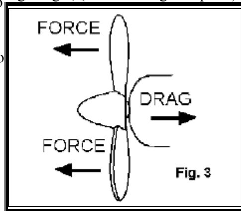
As the plane moves forward, this angle becomes less and less until the plane is moving close to the pitch speed. The actual attack angle will be somewhere in between.
